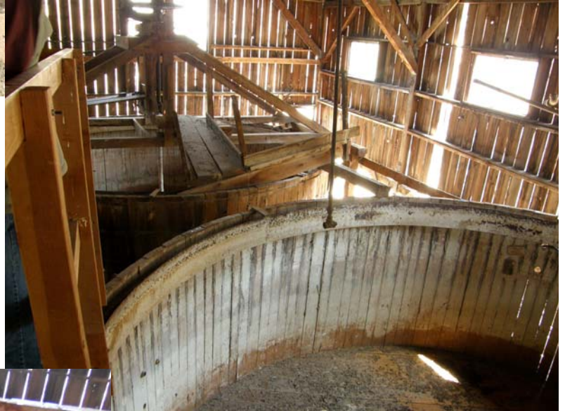
The mixing vats, where cyanide was added to the crushed ore to make a slurry.
