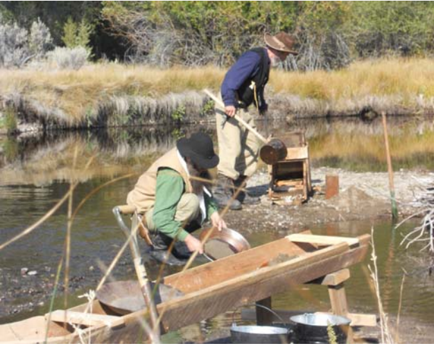
They're still panning for gold in Grasshopper Creek. ABOVE, they have a small sluice and a rocker in operation, whilst, on the RIGHT old fashioned panning.
